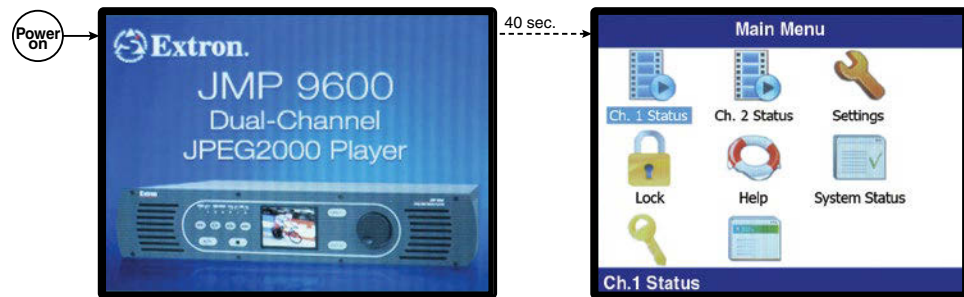
Figure 9. LCD Power up Screen and Main Menu
