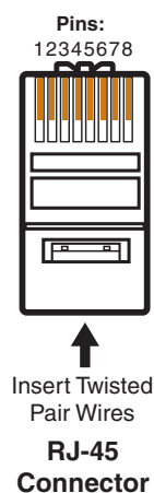
Figure 9. RJ-45 Connector Wiring
