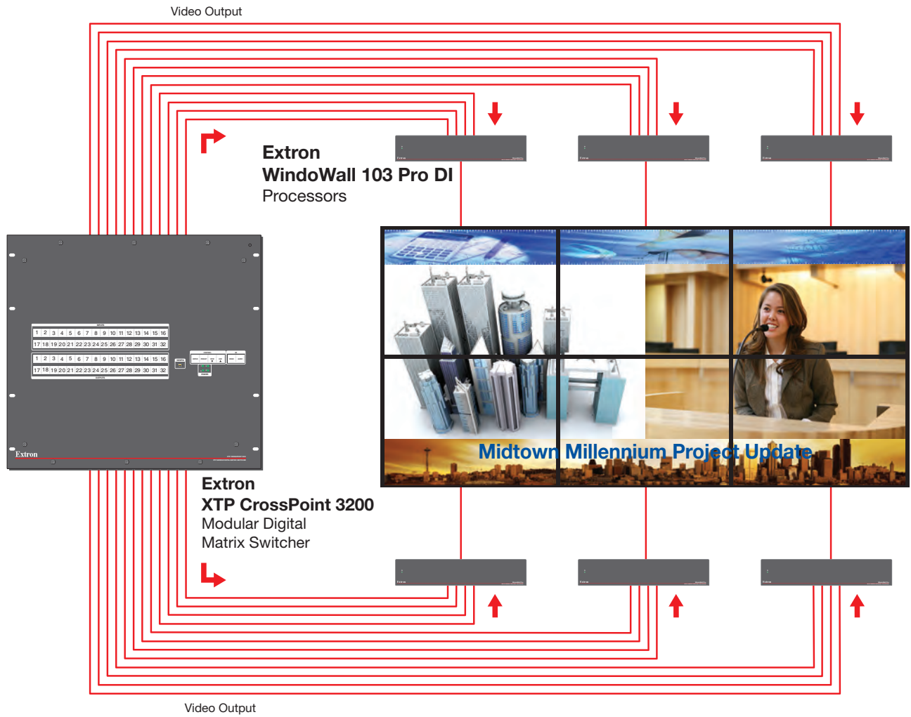
Figure 1. Connection Diagram for a WindoWall Pro DI
