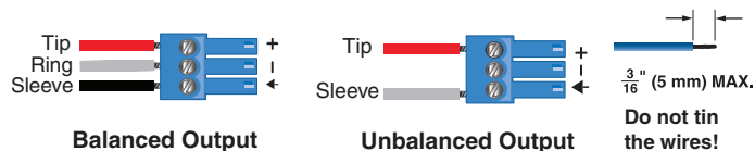
Figure 4. Output Wiring
