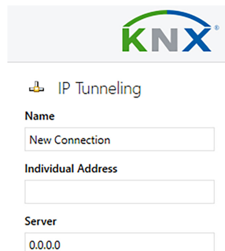
Figure 5. Changing Device Address in ETS
