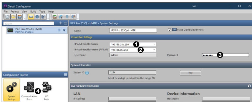
Figure 26. Configuration View — System Settings page for Control Processor
