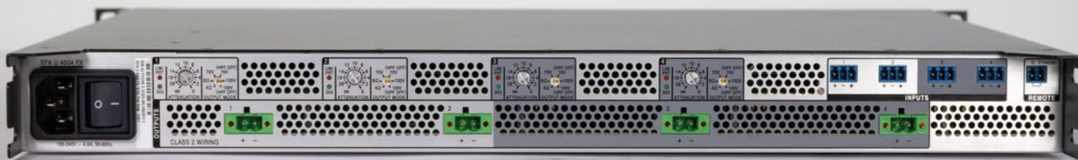
Photo 3: On the back of the 1U housing are the inputs and outputs with two- and three-pin Phoenix connectors as well as the selector switches for the operating mode and the gain controls for the four channels.
