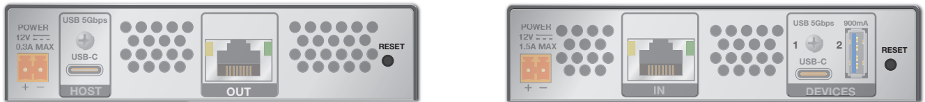
Figure 15. Firmware Reset Button on the UCS T 911 and UCS R 912 rear panels
