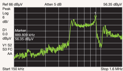
Figure 1 - Variable Frequency Class D Amplifier Output Cable Emissions
