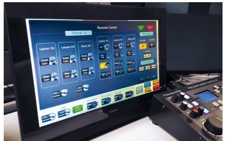
The support team uses an Extron TLP Pro 1520TG TouchLink Pro 15" capacitive touchpanel to manage all AV operations from the control room.
