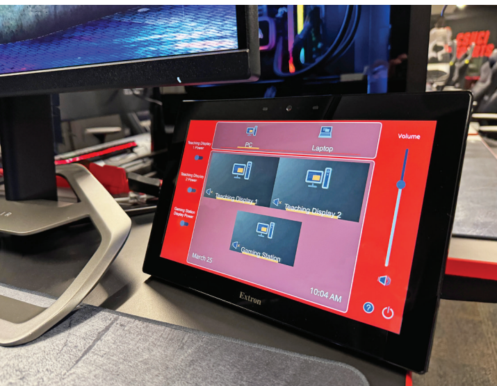
TouchLink Pro touchpanel controls audiovisual content routing to displays, power on/off, and sound volume.
