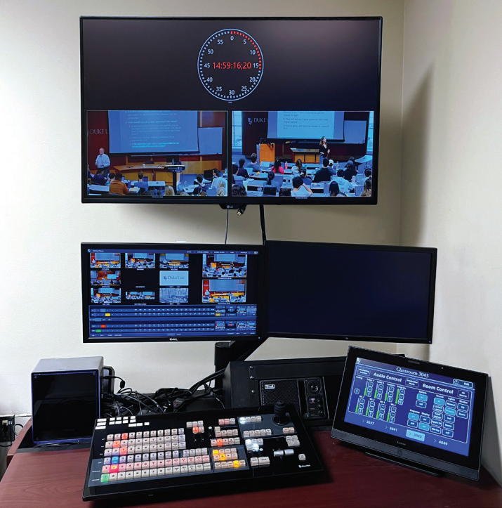
In the control room, a Tricaster control panel and TLP Pro touchpanel put creative options at the fingertips of event producers.
