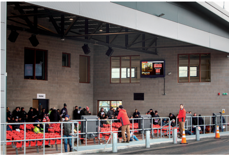
(Left) One of the three auction arenas. Flat screen video displays face bidders from the front ramp, another two displays are on the side walls, and one confidence monitor display is on the rear wall. (Right) Enlarged detail of the confidence monitor display and one of the many speakers.
