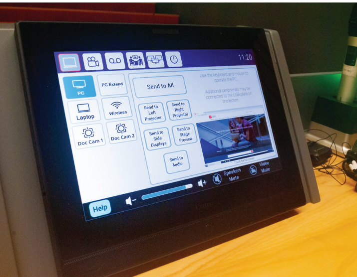
TouchLink Pro touchpanel displays a clear, intuitive AV control interface on a 12" capacitive touchscreen.
