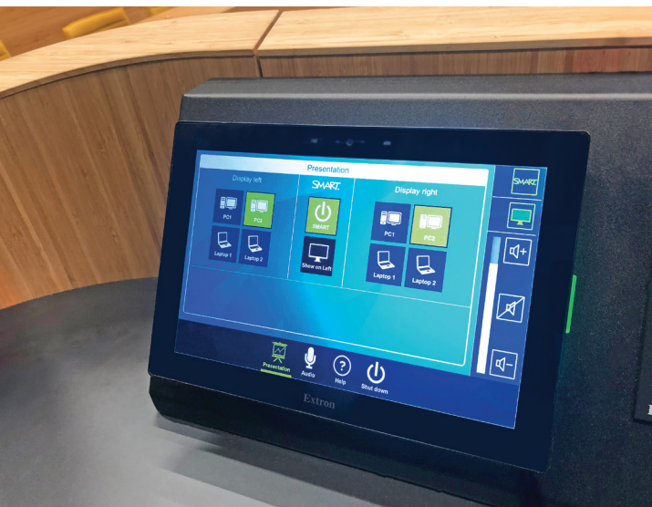
An Extron TouchLink Pro touchpanel makes it easy for instructors to select between various sources for display on the screens in the large lecture hall.
