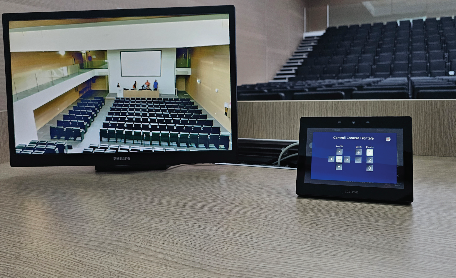
A TouchLink Pro touchpanel at the front of the Aula Magna classroom makes it easy for presenters to control the AV system.
