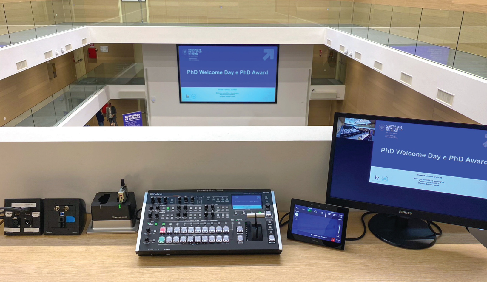
For large events and conferences, an Extron Touchlink Pro touchpanel at the back of the room serves as a central point of control. Photo by Francesco Barreca.
