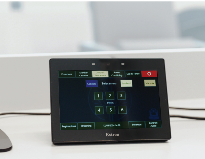
Extron's TLP Pro 725T provides a unified interface for managing AV technology, ensuring flexibility and ease of use for faculty and staff.
