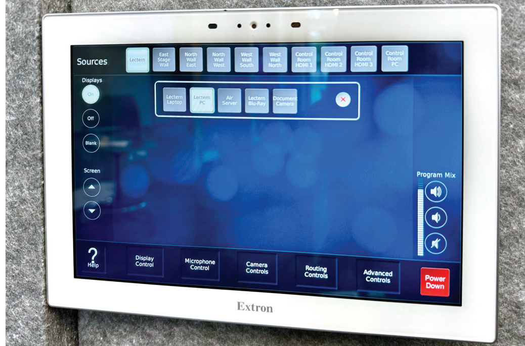
A wall mounted TouchLink touchpanel in the HIP seminar venue.
