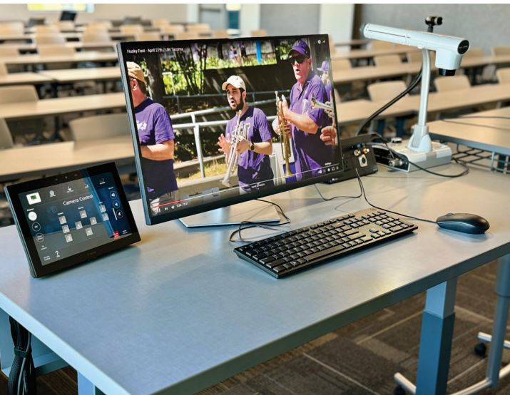
The instructor desks in classrooms 301 and 311 include a PC, document camera, webcam, touchpanel, and auxiliary AV connector panel.
