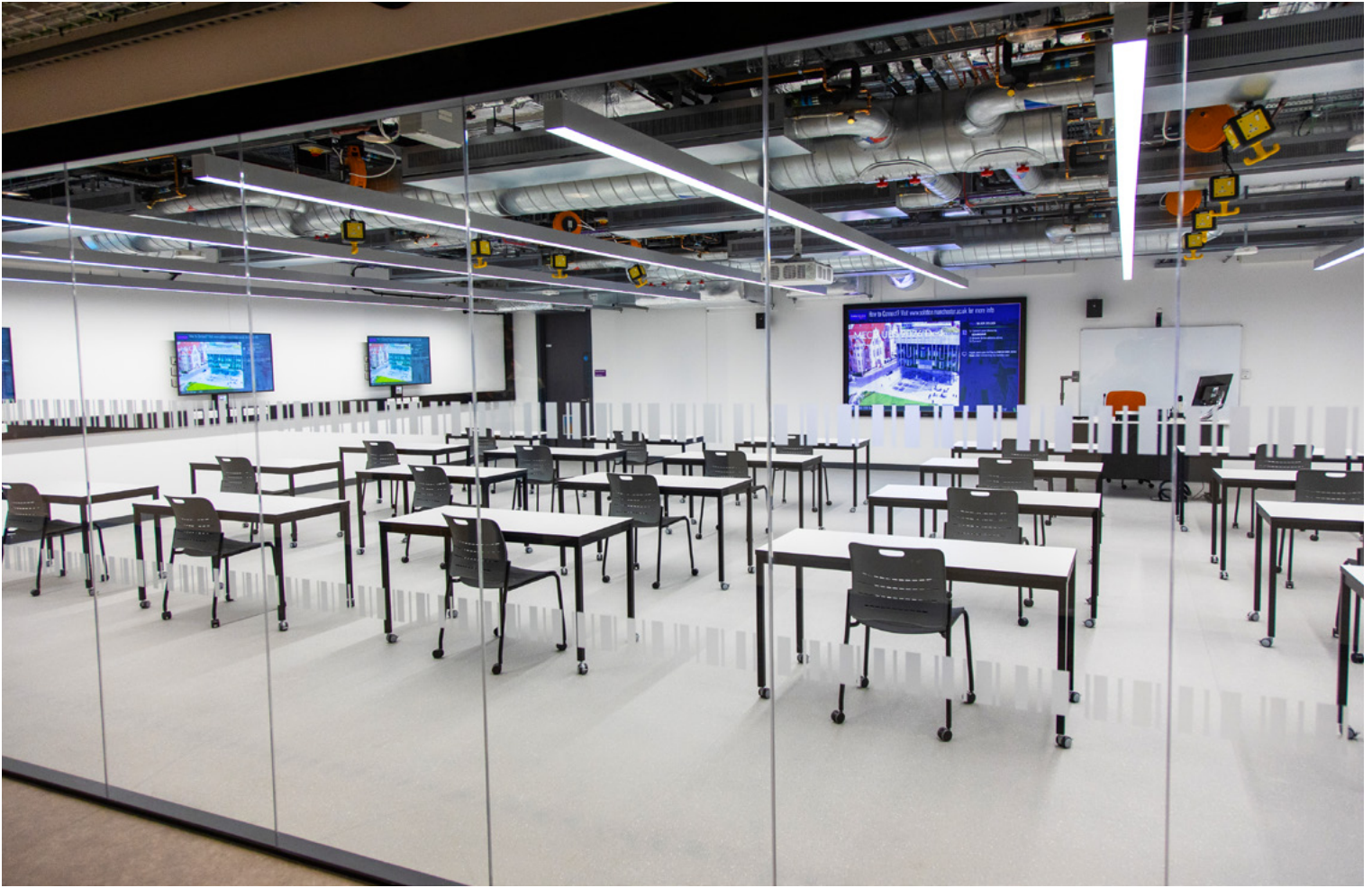
Meet & Teach rooms are designed to be flexible, supporting lecture or collaborative groups. In large and mid-sized rooms, an Extron XTP system or a scaling presentation switcher provides AV signal routing from connected and wireless sources to the multiple displays. Photographs provided by Pure Audio Visual Ltd.
