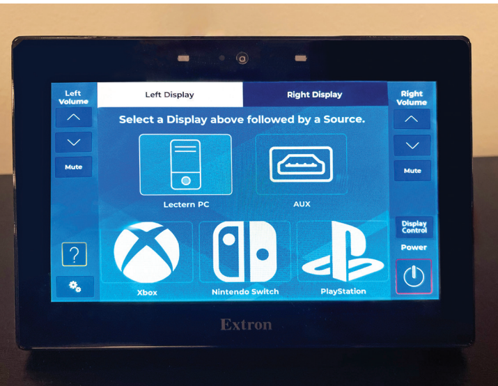
A TouchLink Pro touchpanel on top of the credenza controls routing of the gaming content through the AV system.
