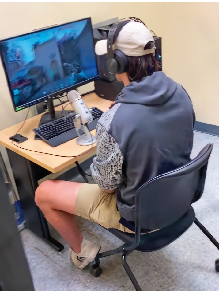
A shoutcaster booth contains a PC for observing play action, a pro announcer condenser microphone, and an audio mixer for combining game audio with play-by-play commentary.
